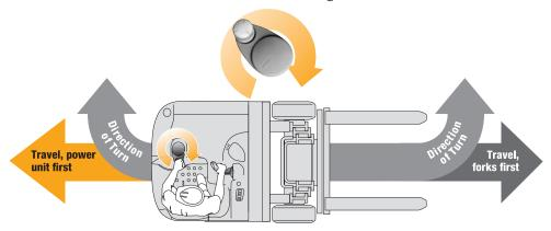
FRONT DIRECTIONAL STEERING (Sometimes called Forward Steering.) Shows direction truck will turn when steering handle is turned clockwise.
