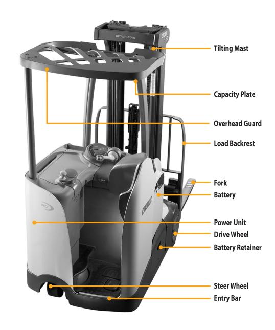
9 Lift Truck Parts Lift Truck Parts 10
