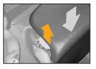
Lift the orange latch at the front of the armrest to release and lower the armrest.
