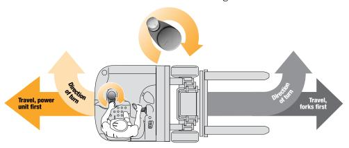
$\begin{tabular}{ll} \bf 2 & FRONT DIRECTIONAL STEERING (Sometimes called Forward Steering.) \\ \bf 2 & Shows direction truck will turn when steering handle is turned clockwise. \\ \end{tabular}$
