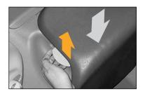
Lift the orange latch at the front of the armrest to release and lower the armrest.
