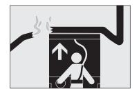
To travel past the cutout height, push the Cutout Override button while, at the same time, pushing either the Raise or Lower button.
