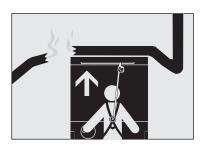
To travel past the cutout height, push the Override Switch while, at the same time, pushing either the Raise or Lower button.
