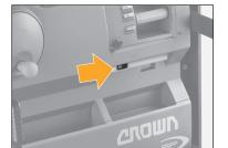
Let go of the pallet by pushing the switch to the right. A light on the switch will illuminate on when the clamp is in the release position.
