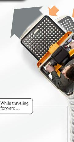
Squeeze the steering control in the direction you want the front of the vehicle to turn. Release the control when the vehicle is turned and pointed to the direction you want to travel.
