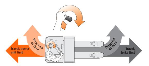
**PRONT DIRECTIONAL STEERING (Sometimes called Forward Steering.)**Shows direction truck will turn when steering handle is turned clockwise.
