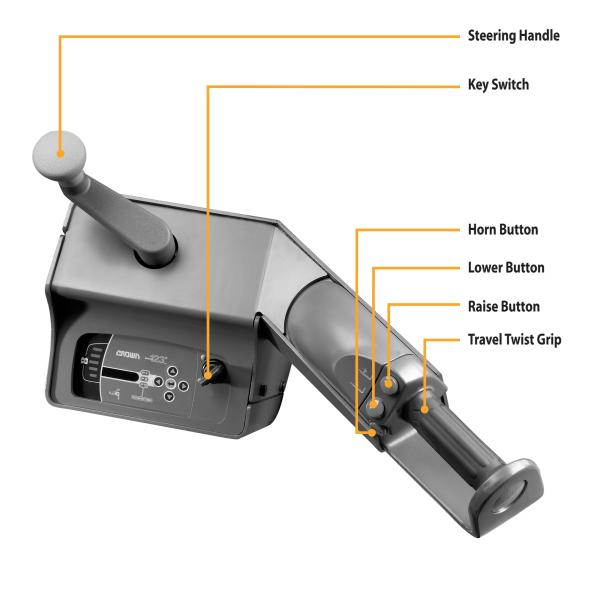
9 Lift Truck Parts Lift Truck Parts 10
