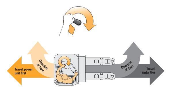
**PRONT DIRECTIONAL STEERING (Sometimes called Forward Steering.)**Shows direction truck will turn when steering handle is turned clockwise.
