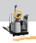
**REAR DIRECTIONAL STEERING (Sometimes called Reverse Steering.)**Shows direction truck will turn when steering handle is turned clockwise.
