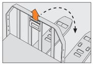
Lift up on the handle and move the backrest forward if you need to service the battery. When you return the backrest to the upright position, make sure the handle is all the way down and the backrest can't tilt forward.
