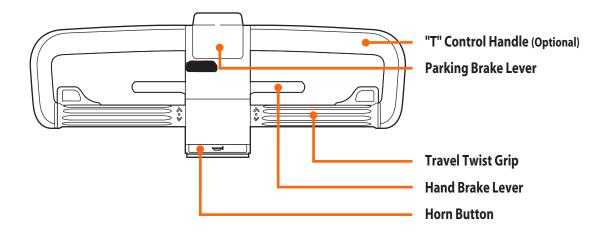
9 Tow Tractor Parts Tow Tractor Parts 10
