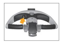
**TO TILT** Push the top of the Tilt switch to tilt the tip of the forks up. Push the bottom of the Tilt switch to tilt the tip of the forks down.
