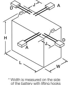
Connector Location / Length (J): A/15" (A/381mm) for all battery sizes except 80 Volt "D" Batteries require D/22" (D/559 mm).
