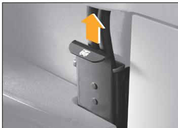
Use the power disconnect to shut the truck down any time it isn't working right. Don't use the truck if it's not working right. Report the problem to your supervisor.
