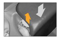
Lift the orange latch at the front of the armrest to release and lower the armrest.
