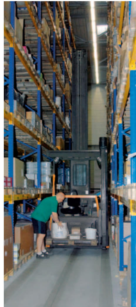
Only the TSP 6000 allows operators to exit the cab in an aisle in order to pick items from the lowest level.
