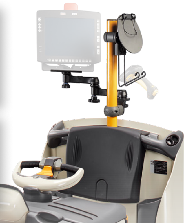
Rear tube with small clip pad, scan gun holder and adjustable arm for WMS monitor
