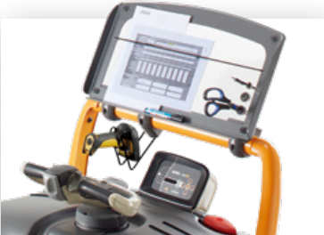
Front tube with large, see-through clip pad and scan gun holder
