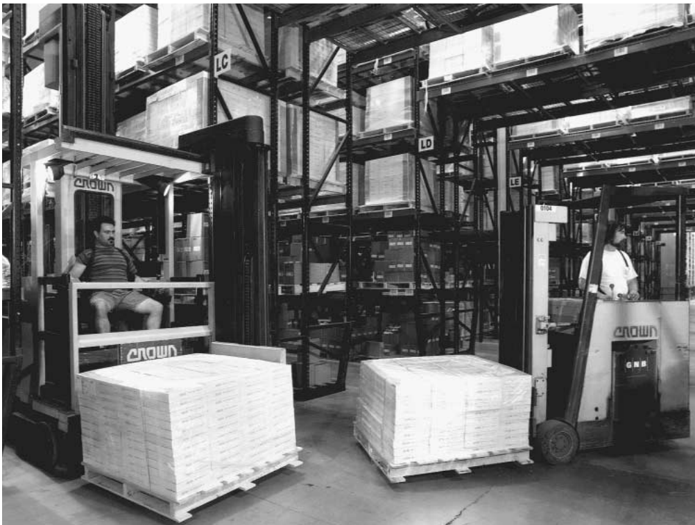
Crown Series TSP Turret Stockpickers and Series RC stand-up riders are shown above working together in storing and retrieving a variety of aftermarket brake products. Brake Parts, Inc., ships up to 800 pallets of merchandise daily from their McHenry, IL, distribution center.
