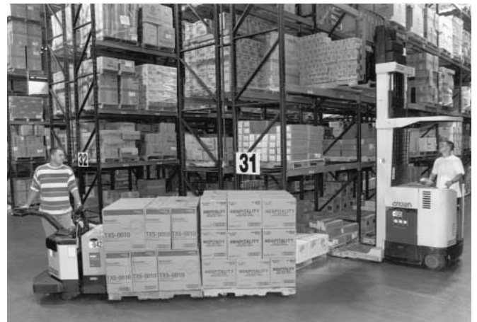
The Crown PE 3000 Series Rider Pallet Trucks with double pallet capabilities are important in moving various products to-and-from staging areas. Above, the double pallet truck works with a Crown reach truck in Mutual's dry storage area.
